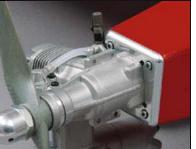
The specially designed aluminum engine mount accepts virtually any engine in the Viper 500's recommended range. A fuel tank and generous package of Great Planes' quality hardware are also provided
