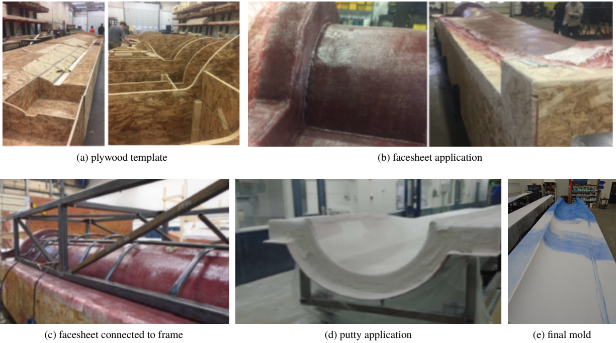
Fig. 9 Fabrication of the blade molds.
