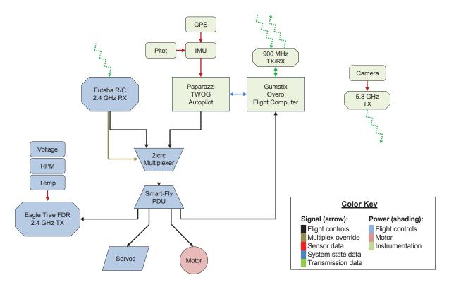
Figure 11. A flowchart diagram of the avionics suite showing a top-down view of flight control signals, multiplex the override command signal, sensor inputs, instrumentation communication, and transmission routes.
