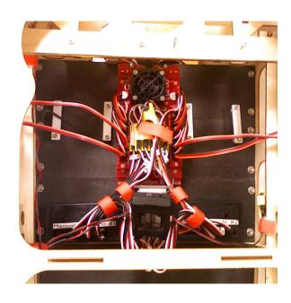
Figure 7. Smart-Fly power distribution unit, JR receiver, and 2irc manual overrides installed on the front balsa/carbon-fiber sandwich tray.
