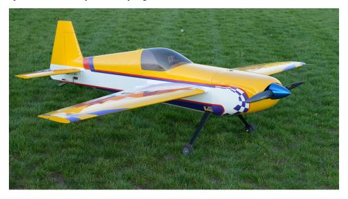
Figure 1. A photograph of the UIUC Aero Testbed, which is an electric unmanned 35% scale Extra 260 aerobatic aircraft with a 105 in wingspan, a weight of 37 lb, and is instrumented with an avionics suite that includes a 6-DOF inertial measurement unit, GPS receiver, and pitot probe among other sensors.
