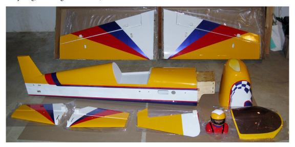
Figure 6. All major airframe components that arrived with Hangar 9 35%-scale Extra 260 ARF kit.
