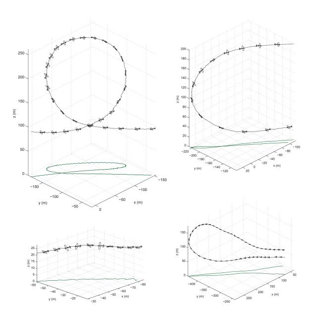
Figure 13. Trajectory and ground trace plots of aerobatic maneuvers, starting on the top left and going clockwise: a) loop, b) Immelmann, c) roll, and d) half Cuban-eight.
