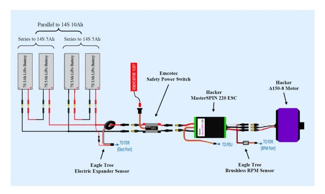
Figure 8. A propulsion system diagram for the Aero Testbed unmanned aircraft.
