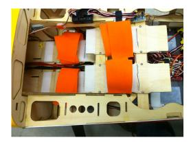
Figure 10. A photograph on the motor battery trays where the Eagle Tree Systems Flight Data Recorder can be seen at the top of the shot.
