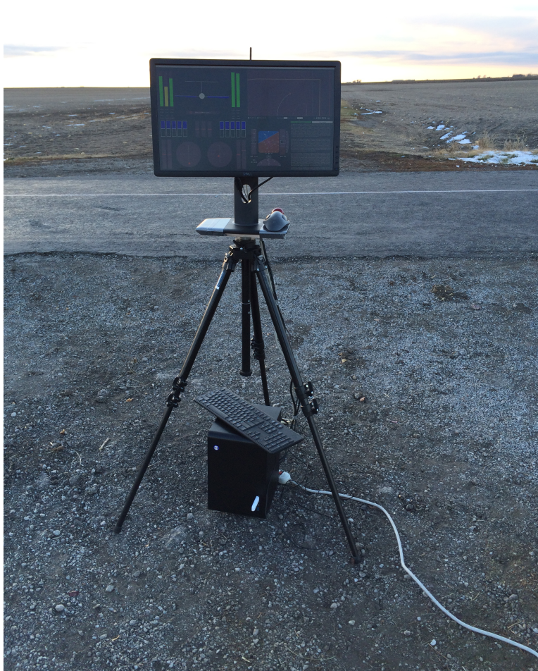
Figure 5. A photograph of the sensor data acquisition system unmanned aerial system (SDAC-UAS) ground interface during flight.
