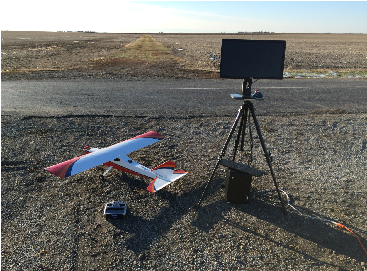
Figure 1. A photograph of the entire system used in the test implementation of the SDAC-UAS: the aircraft instrumented with an SDAC (internal - not visible) and ground interface.
