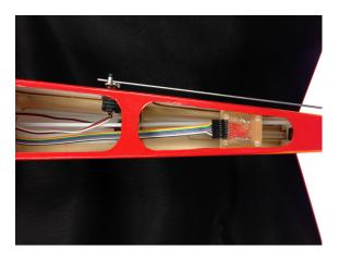
Figure 9. Bottom view of the tail with the coating removed showing the elevator and rudder potentiometers and standalone magnetometer installed.
