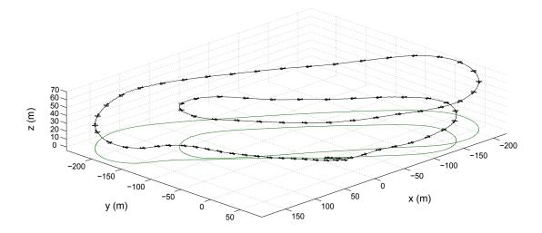
Figure 16. Flight path for initial test flight (the aircraft is drawn three times bigger than the actual size and once every second tangent to the flight path).
