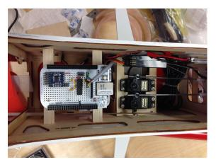
Figure 7. The sensor data acquisition system installed into the fuselage.
