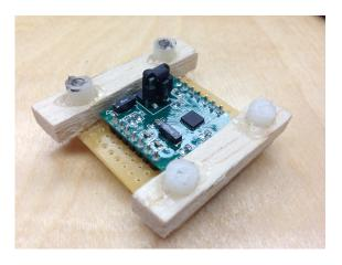
Figure 8. The stand-alone magnetometer on the perfboard mount before installation.
