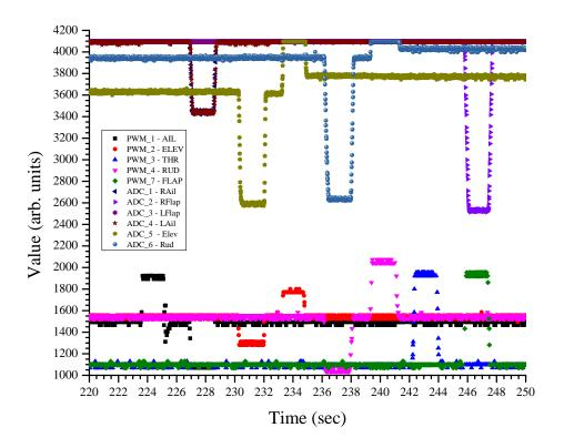
Figure 15. Recorded control inputs and potentiometer measured deflections.
