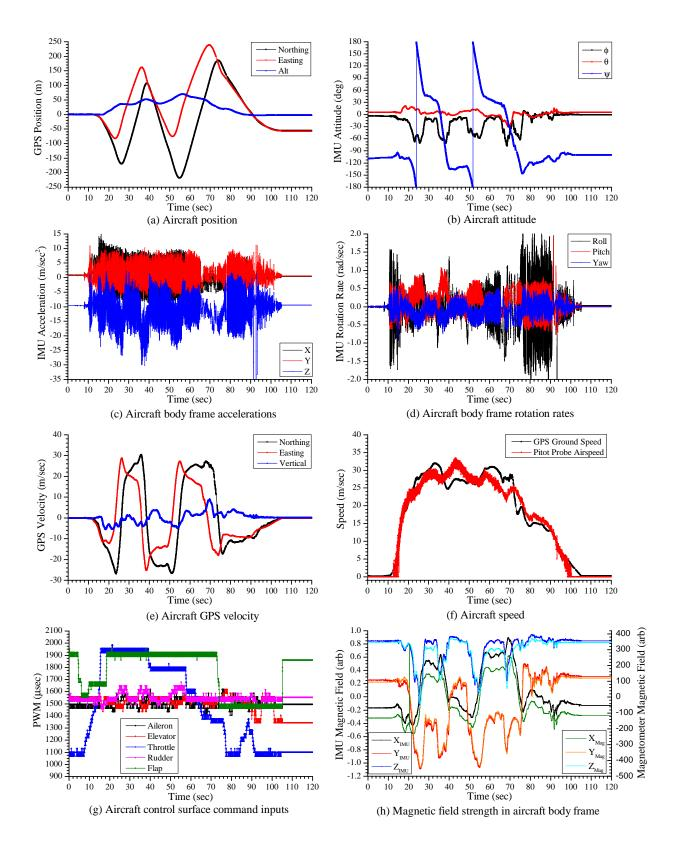
Figure 17. Sensor outputs for initial test flight.
