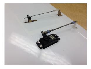
Figure 12. Completed view of the left aileron servo and potentiometer setup with all the linkages installed.
