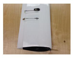
Figure 13. Outboard section of the left wing with the pitot probe, aileron, aileron servo, and aileron potentiometer system in view.
