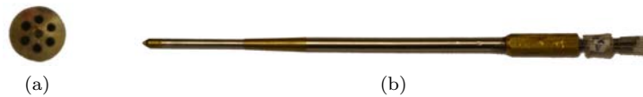
Figure 2: Photographs of the Aeroprobe 7-hole probe used during testing: (a) front view and (b) side view.
