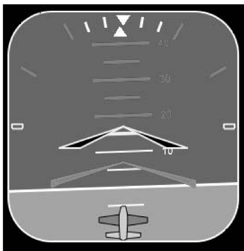
Fig. 22 Envelope protection warning that aircraft is nearing unsafe attitude (pitch down command).
