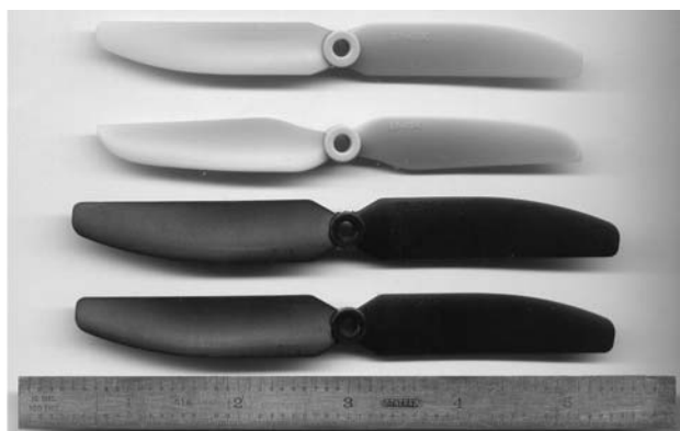
Figure 3. GWS Direct Drive propellers with diameters of 4.5 in. and 5.0 in.
