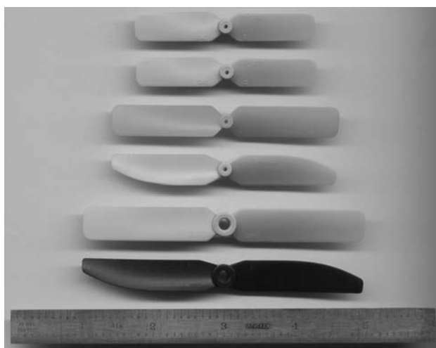
Figure 2. GWS Direct Drive propellers with diameters ranging from 2.5 in. to 4.0 in.
