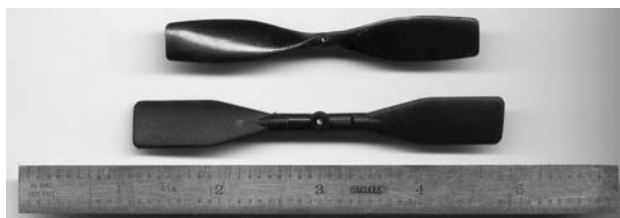
Figure 7. Union propeller with a diameter of 3.15 in. and KP Aero Models propeller with a diameter of 3.8 in.
