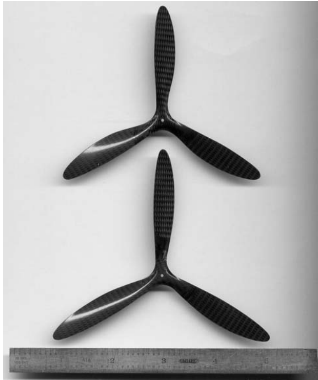
Figure 5. Micro Invent 3-bladed propellers with diameters of 4.3 in. and 5.0 in.
