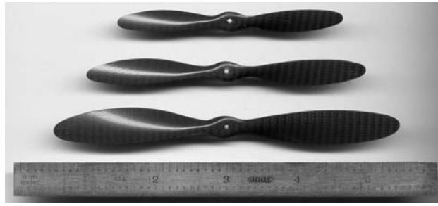
Figure 4. Micro Invent propellers with diameters ranging from 3.2 in. to 5.0 in.
