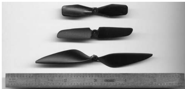
Figure 6. Plantraco propellers with diameters ranging from 2.25 in. to 4.0 in.
