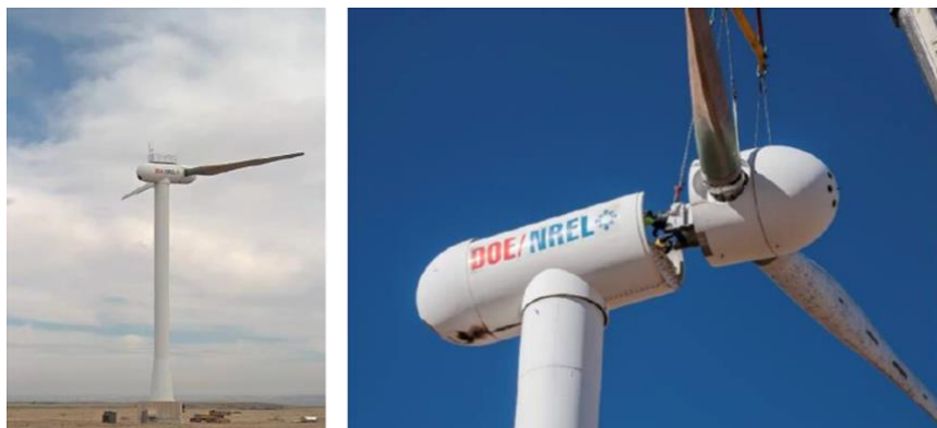
Figure 2. SUMR rotor on CART2 with 12.5° coning (credit NREL)
