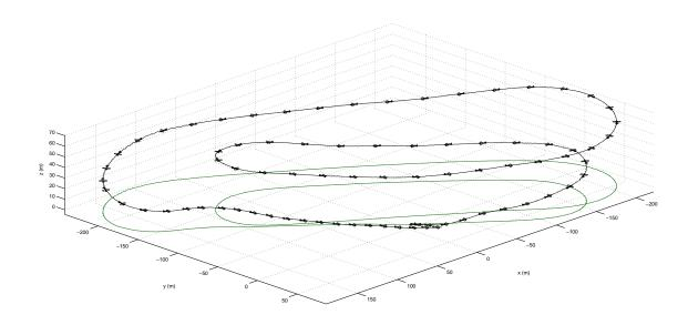
Fig. 5. Flight path. The aircraft is drawn three times bigger than the actual size and once every second tangent to the flight path.
