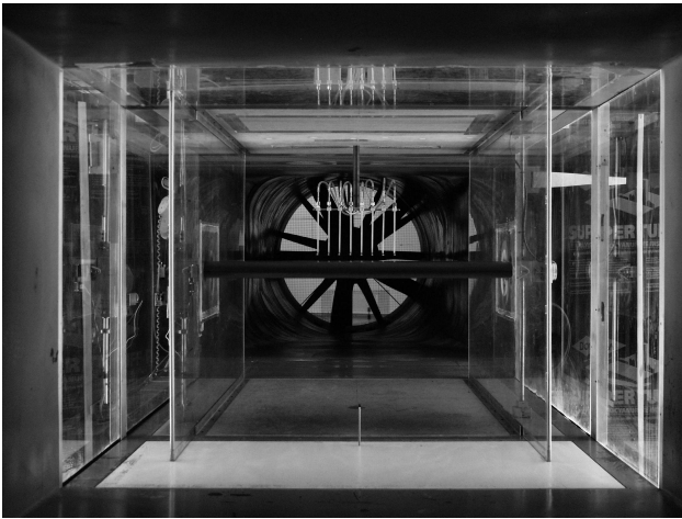
Fig. 1 Photograph of wind-tunnel test section with model, splitter plates, and vertically-traversed wake probe array installed.
