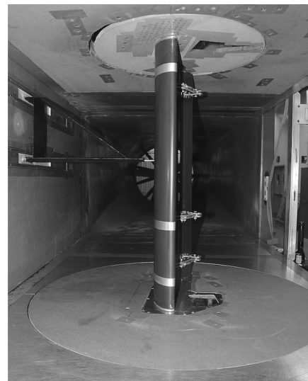
Fig. 6 Experimental setup of sidewall-mounted traverse with three-element airfoil model installed.
