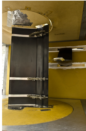
Figure 5. Sidewall-mounted traverse setup for current test.
