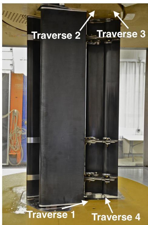
Figure 6. Location of four traverses relative to wind tunnel model.
