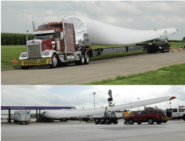
FIGURE 11.1 Photograph of wind turbine blade being transported by road (Top) and refueling of a blade-carrying truck (Bottom) in Walcott, Iowa.
