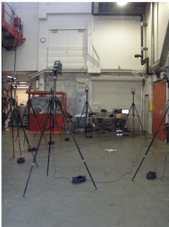
Figure 1. Motion tracking facility using the Vicon system at UIUC.
