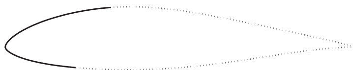
Figure 4. Position of the wind protection tape (bold line) on the DU 96-W-180 airfoil ending at x/c = 30\% on the upper surface and x/c = 20\% on the lower surface.
