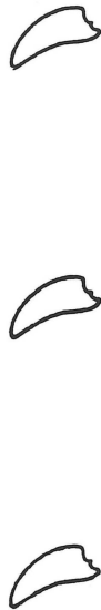
Figure 3-19 Example cascade derived by the inverse method without Newton iteration ( K_H = 7.652 , \bar{K}_H = 8.656 ).
