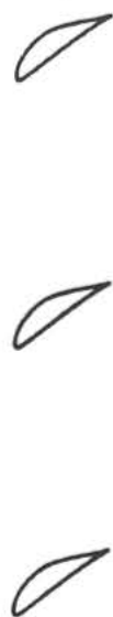
Figure 3-20 Example cascade designed by the inverse method with Newton iteration ( K_H = 0.25 , \bar{K}_H = 0.25 ).
