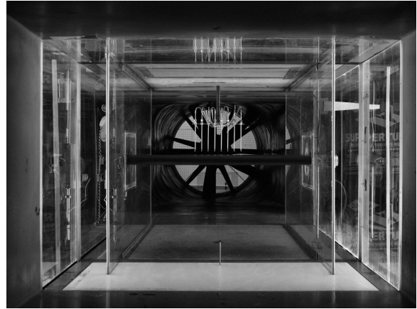
Figure 8: Photograph of the UIUC 3×4 ft low-speed subsonic wind tunnel test section.
