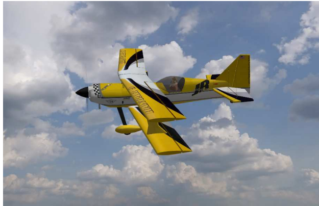
Figure 27. 46%-scale Ultimate TOC biplane used in simulations [rendering taken from simulator, wingspan of 2540 mm (100 in)].
