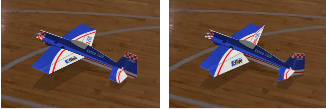
Figure 1. Extra 260 ultra-agile aerobatic foam-construction electric propeller-driven RC aircraft with large control surfaces at neutral and maximum deflections [wingspan of 826 mm (32.5 in)].
