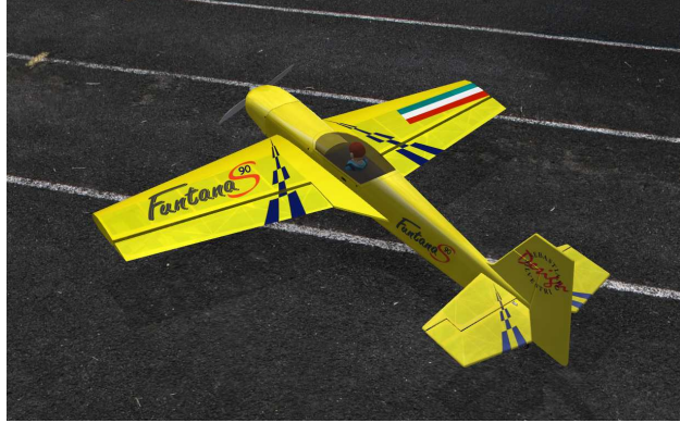
Figure 10. Funtana 90 used in simulations [rendering taken from simulator, wingspan of 1765 mm (69.5 in)].
