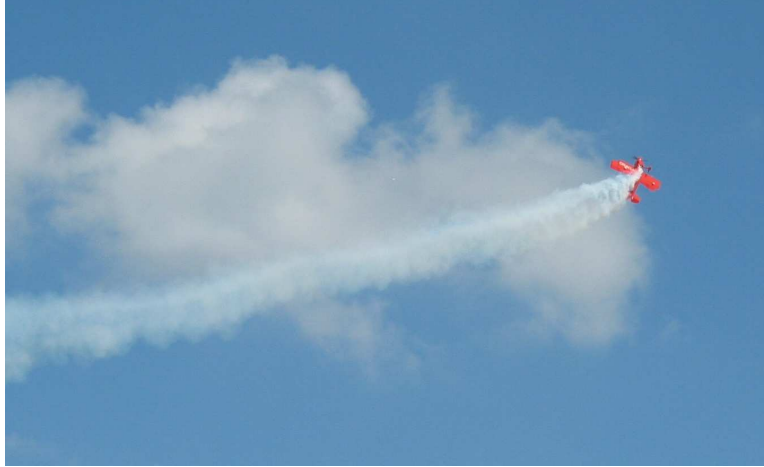
Figure 8. Sean Tucker performing a knife edge slide aerobatic maneuver with airshow smoke that shows strong propeller wash streaming along fuselage right side (aircraft bottom surface is to the camera).
