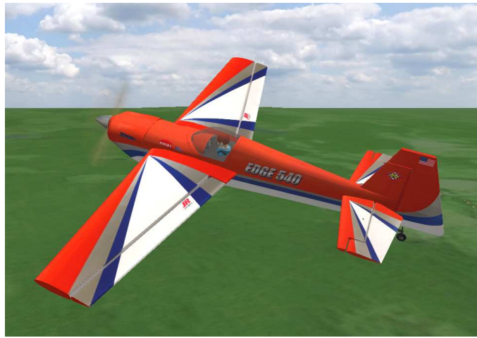
Figure 1. 33%-scale Edge 540 aerobatic RC model used in the simulations.
