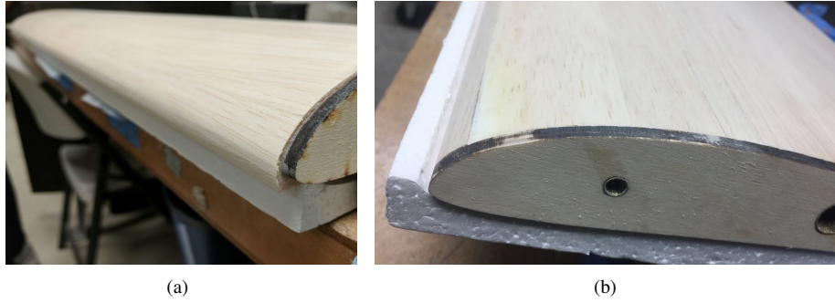
Figure 7. VASI715 model construction: (a) before sanding (b) after sanding
