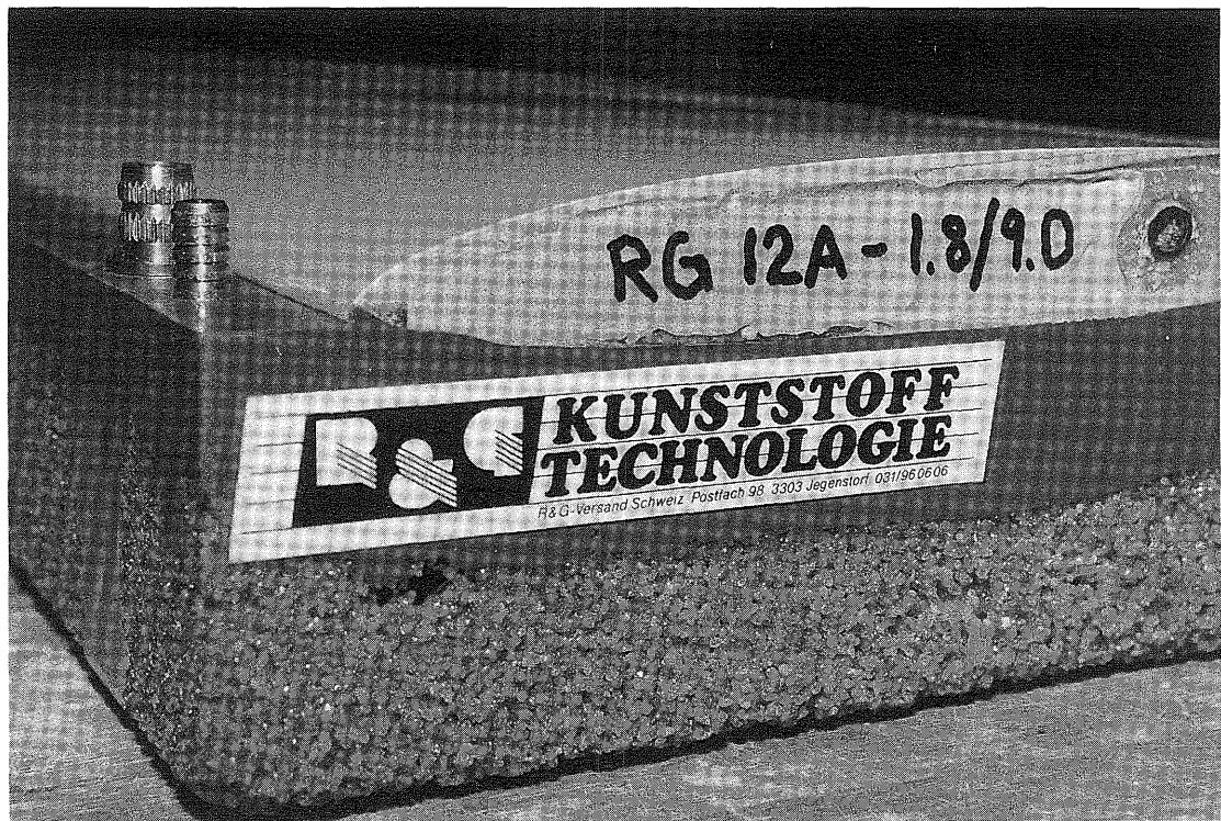
Figure 9: Close up of the lower half of the mold. Clearly visible is the positioning bolt and nut to pull the halves together in the molding process. The airfoil used is RG 12A-1.8/9.0.
