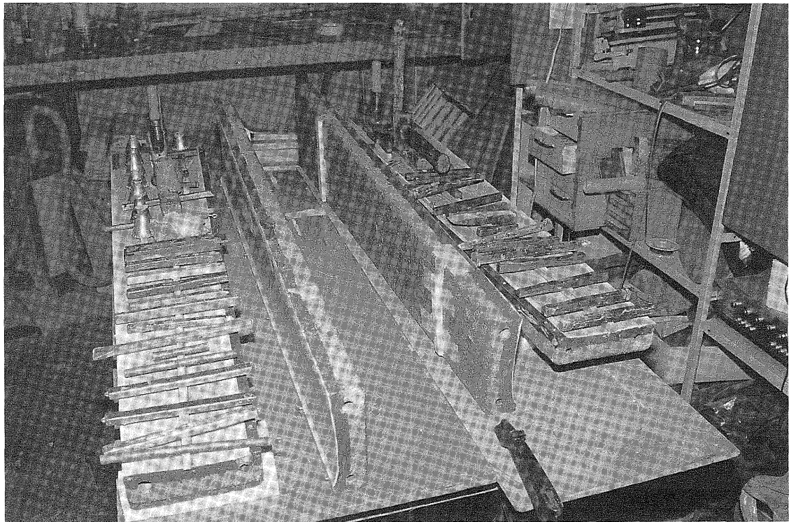
Figure 17: The main spar and auxiliary spars (consisting of roofmate foam which in the USA is more commonly known as Styrofoam or blue board) are being glued to the lower moldings of both wings with epoxy resin. Lead weights are used to press the spars down tightly to the skin moldings.
