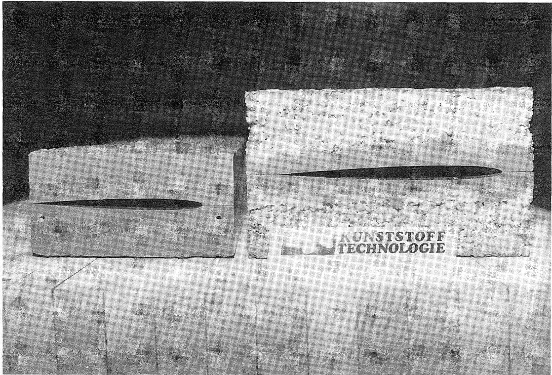
Figure 33: The finished horizontal tail molds of the smaller "Speedo 84" model on the left, and the "Speedo 87" model on the right.
