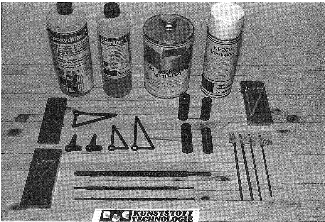
Figure 41: Parts especially molded for the "Speedo '84 and '87" projects. The plastic bottles on the left contain the LF epoxy resin and hardener. The metal can on the right contains R+G liquid wax separating agent and the can with the white cap is R+G sprayable release agent used for hard to get to corners which is especially useful for the small lever molds.
