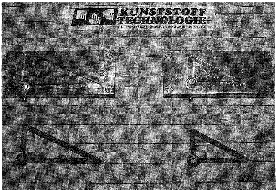
Figure 50: The elevator molds with their respective finished levers.
