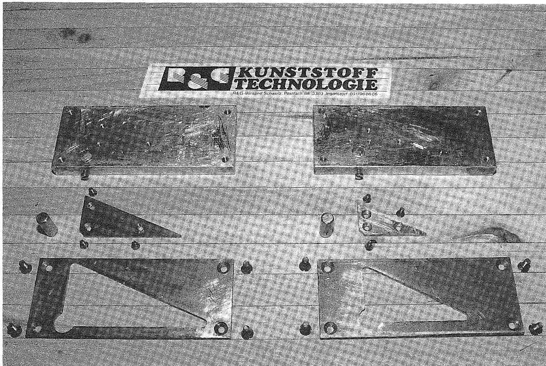
Figure 46: The elevator lever mold; each consisting of four main parts. This has been machined and milled from aluminum and steel.
