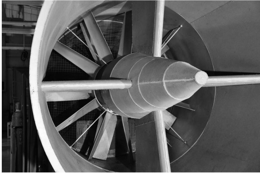
Figure 3.3: Photograph of wind tunnel fan and stators.
