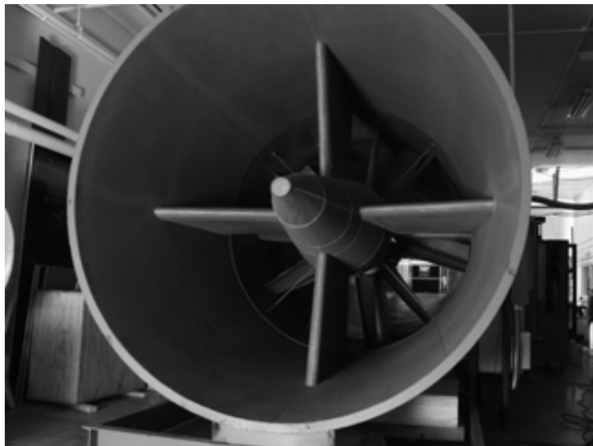
Fig. 2.3 Photograph of wind-tunnel exit fan.
